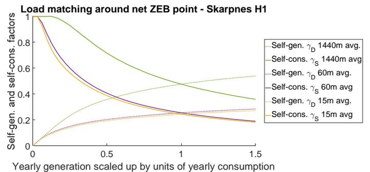
Figure: Effect of resolution on load matching factors at net ZEB point Økern (upper) and Skarpnes (lower)
