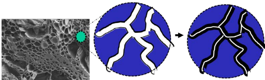
Figure 5: Porous biocarbon can be blocked by depositing carbon in its pores.
