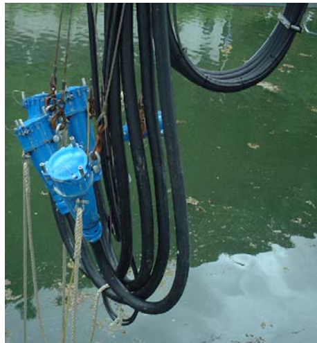
Figure 1 A typical power line connector, which is used today
