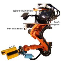
Fig. 3. KUKA robot manipulator hanging upside down from the Güdel gantry. The structured light vision system is mounted on the base and the sensor lid operation tool is mounted on the end effector.
