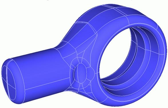
Example: Patch structure of a fairly simple CAD-object
