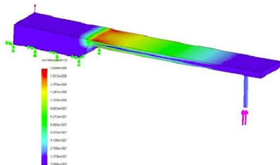
Figure 2: FEM simulation of cantilever design. Red color indicates area with high stress concentration
