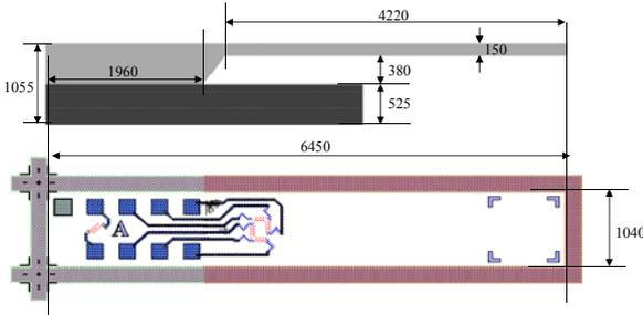
Figure 3: Outline of the Si/glass cantilever die with a Wheatstone bridge and a fifth resistor for temperature compensation.
