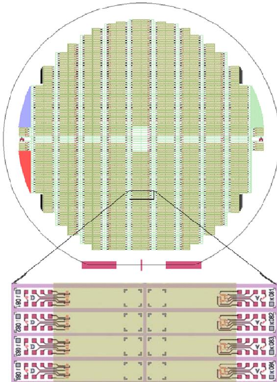
Figure 4: Wafer design showing the die distribution on the wafer.
