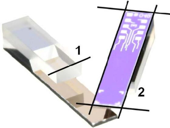
Figure 5: Illustration of the multi-step dicing process of the silicon-glass stack for release of individual units
