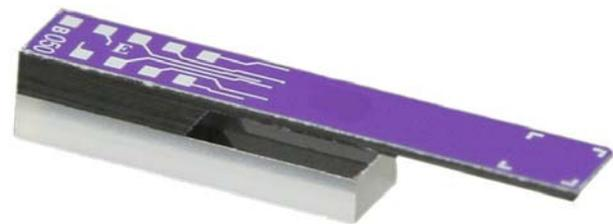
Figure 1: A piezoresistive silicon/glass cantilever die for position sensing
