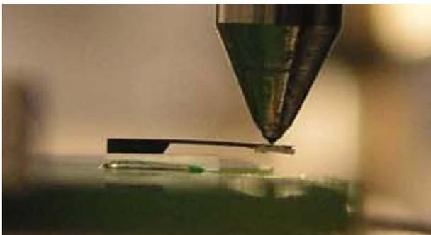
Figure 6: Test of mechanical strength of an assembled cantilever component
