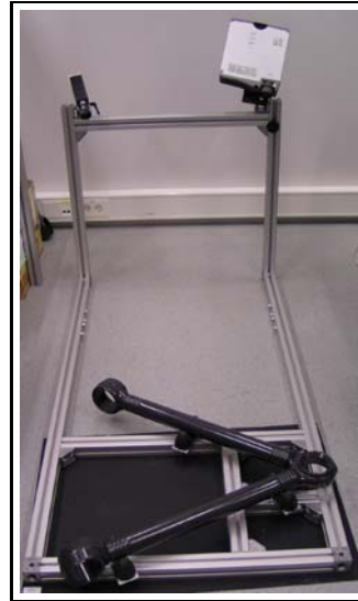
Figure 4. Measurement cell for inspection of V-stay
