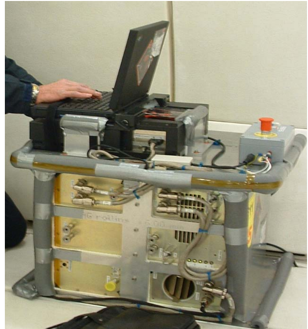
Fig. 6 Compact and sheltered ANITA set-up for the submarine test measurements
