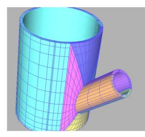
Spline space refined to have matching lines in each hexahedral NURBS-block to produce a watertight representation
