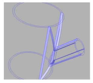
• The internal faces produced by the splitting process
