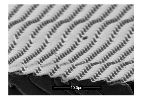
Left: Scanning electron micrograph showing the surface patterning on a part of a DOE. Diffractive optical elements can perform several key functions such as dispersion, focusing and beam splitting in instruments for spectroscopy [2].
