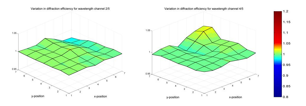
Simulations for a four-level silicon grating coated with 30 nm of gold. This profile shows less of the resonances that we see for the two-level profile above.
