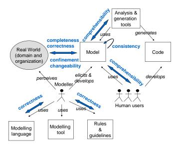
Fig. 7. Model quality goals in MBSD with transformation of real world to running software
