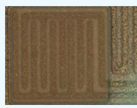
Finger electrode width/gap 150/100 µm.
