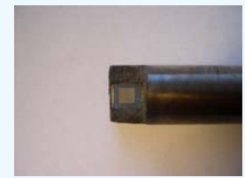
Finger electrode, resistive sensor.
