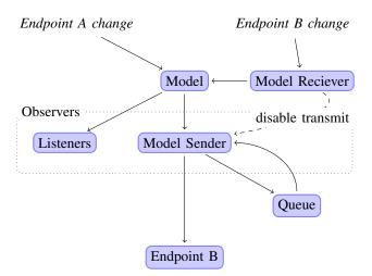
Fig. 3: The Event Loop of a Tinia Application. Conceptually the same event loop is executed both on the client and the server.
