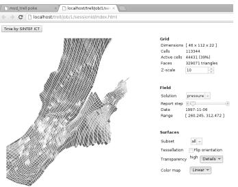
Fig. 4: A reservoir visualization web-application, allowing for loading and navigating massive datasets on demand. The GUI is automatically generated by the framework.
