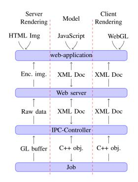
Fig. 2: Component communication diagram, illustrating how each component encodes and decodes the various content streams.
