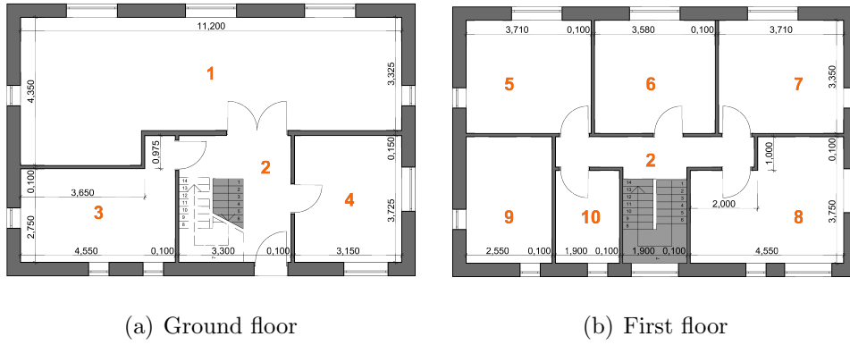
Figure 1: Sketches of the ground and first floors : kitchen coupled to the living-room (zone 1), corridor with an open staircase (zone 2), laundry (zone 3), office (zone 4), four bedrooms (zones 5 to 8) and a bathroom (zones 9-10). The south direction is pointing upwards.
