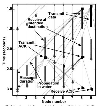
Clock time (seconds) downwards. Node numbers (1-9) horizontally. The diagram shows message transmission, duration, propagation and reception. Original colour coding not visible here shows collisions and special events.
