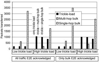
Low trickle load is around 7% of capacity (sum of all sources). High trickle load is 45% of capacity Trickle traffic shown alone, combined with one multi-hop bulk transfer and combined with one single-hop bulk transfer. Figure 8. Trickle load and bulk transfer
