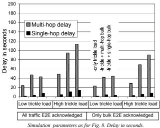
Figure 9. Bulk transfer influence on trickle flow delay
