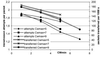
Bulk transfer of data from node 14. Fixed rate unacknowledged traffic (~40% of capacity) from all other nodes. Slot time=0.1s. Fair queuing. Figure 5. Effect of CWmin and CWmax
