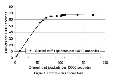
In the next scenario simulated a window based transport layer flow control protocol has been added. One data flow is set up from each node towards the master. The master uses the window mechanism to constrain all flows to the same rate. This mechanism is equivalent to polling from the master with several active polls in the network at the same time.
