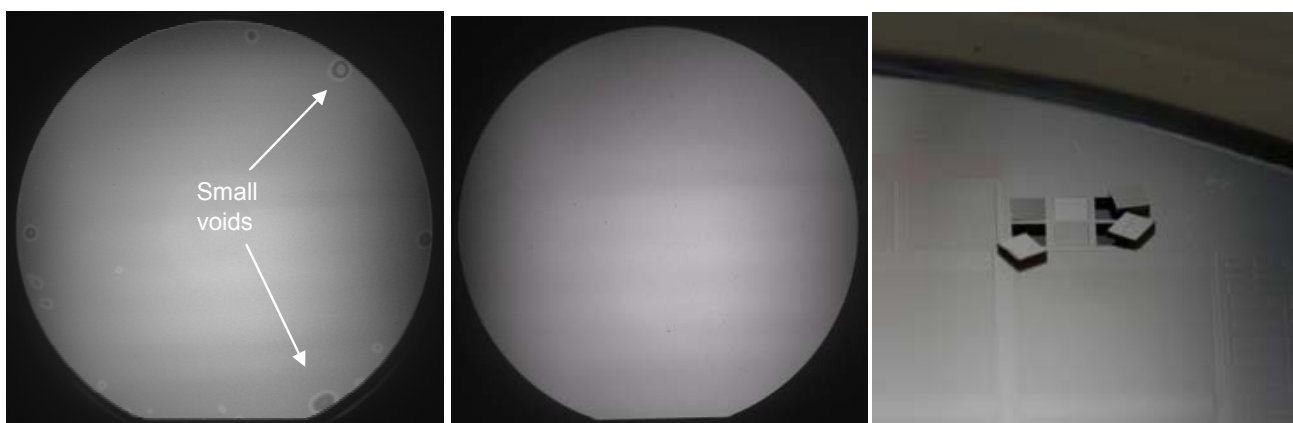
Fig.6a (left): Small voids were observed before annealing. Fig.6b (centre): The wafer appeared to be perfectly bonded after 2 hours of annealing at 1050°C in nitrogen. Fig.6c (right): Detectors detached from the bonded wafer where bonding was poor.
