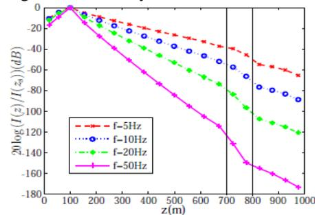
Fig. 1. Current distribution along the wire antenna at different frequencies.
