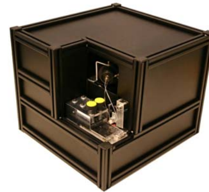
NASBA amplification & detection instrument
