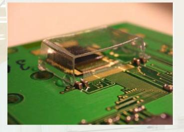
One module successfully recorded particles from an Am-241 source
