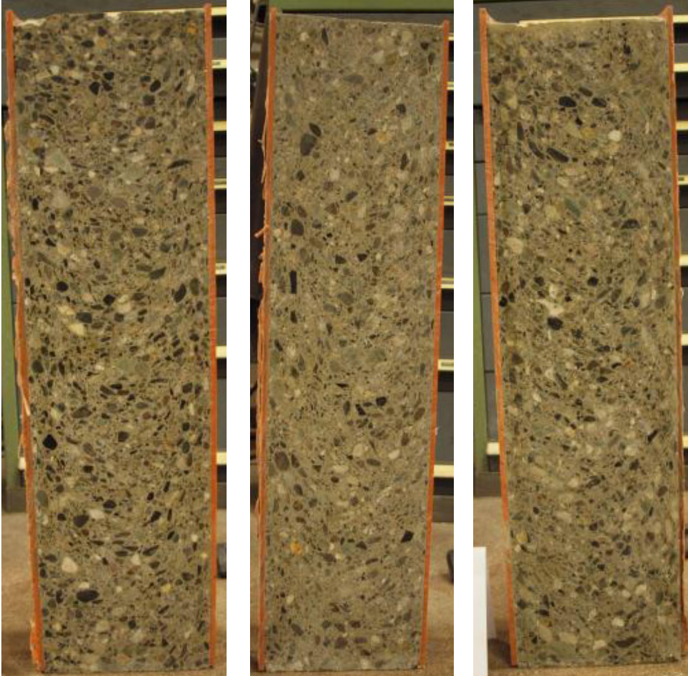
Figure 11: The cross sections of the hardened concrete cylinders; from left to right: unstable SCC, filler stabilized and chemically stabilized.
