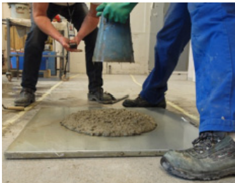
Figure 2: Slump flow and T500 measurement.
