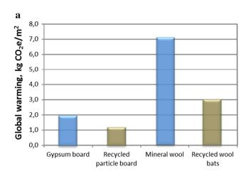
Fig. 2 Contribution to global warming from material recovery of C&D wood waste according to LCA results. **a** Attributional LCA: Production of 1  $m^2$  "traditional" board or insulation bats (*blue bars*) and 1  $m^2$  particle board and insulation bats made of recovered C&D wood waste (*brown bars*), **b** Consequential LCA: Material recovery
