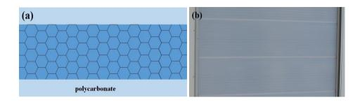
Fig. 3. (a) Schematic drawing of commercial aerogel glazing product shown in pane (b). Aerogel granules are contained in the honeycomb arrangement of cells.
