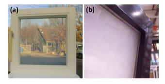
Fig. 1. (a) Specular [14] and (b) diffuse [10] aerogel glazings/windows.
