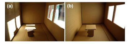
Fig. 2. Comparison between (a) specular double glazing and (b) diffuse aerogel glazing for daylight management by using a cardboard house model [8].
