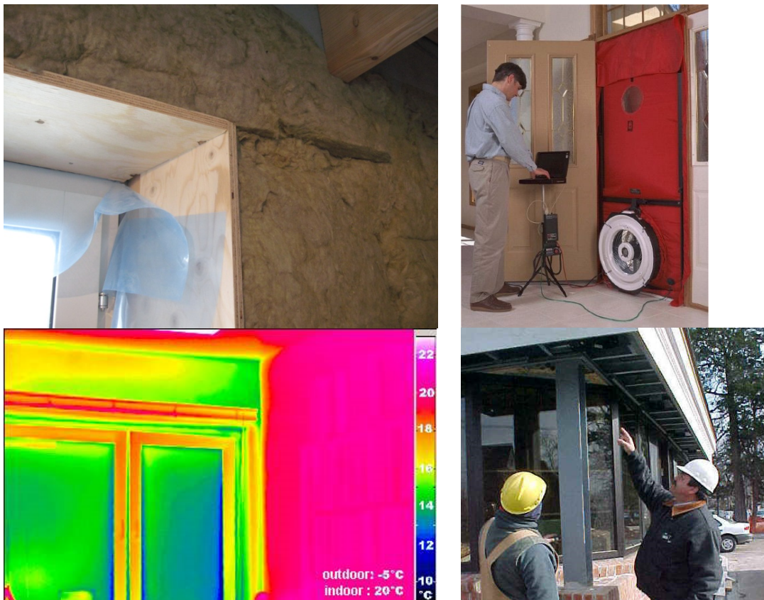
Figure 7.1: Site visit at passive house project in Uddevalla, Sweden (top left); Blower door test (top right); Thermograph of window and wall (bottom left), visual control site visit (bottom right) (Photo: SINTEF Byggforsk; draftstop.net; passivhaustagung.de; hartford.gov)
