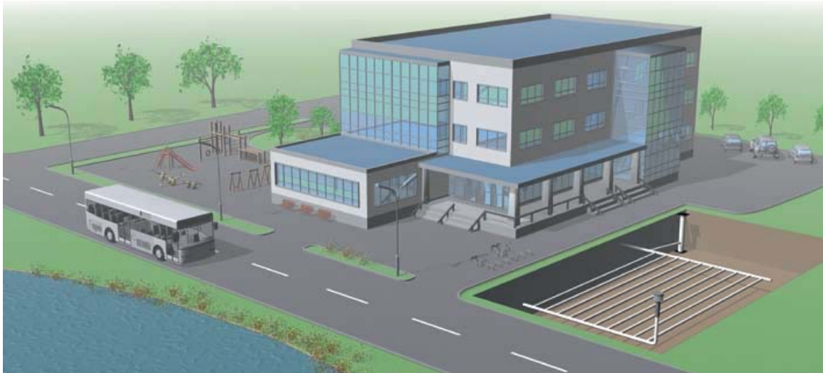
Figure 3: ETAHE with several parallel pipes (Source: Rehau)
