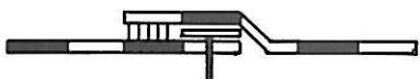
Fig. 11. Single-ply membrane with fastener at edge of felt and full bonding outside edge of stress plate
