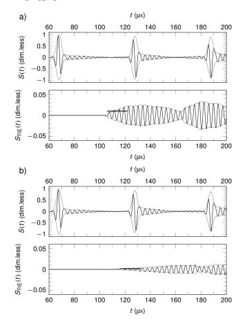
Figure 7: Received full signal and extracted TIE signal from the cases shown in Figure 6 of  $30^{\circ}$  transducer angle and eccenterings of a)  $\epsilon = 9.40$  mm and b)  $\epsilon = 18.80$  mm.
