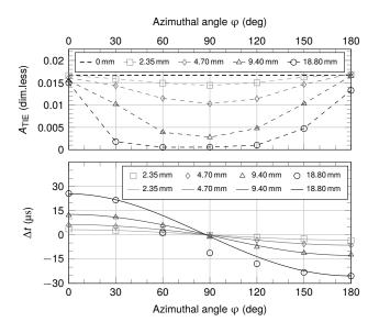
Figure 8: Upper: RMS amplitudes of TIE signals as per Equation 3 against casing 2 eccentering  $\epsilon$  and transducer angle  $\varphi$ . Lower: Additional TIE propagation time against eccentering and transducer angle, both from simulations (marks) and from Equation 5 (lines).
