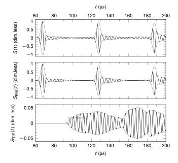
Figure 3: Received signal and its envelope for the full model (upper) and for the auxiliary model (middle). Both models are shown in Figure 2. The TIE signal found as the difference of the two signals is shown in the lower plot, with a black bar that indicates the representative TIE RMS amplitude  $A_{\text{TIE}}$  (Equation 3) and the period over which it was determined.
