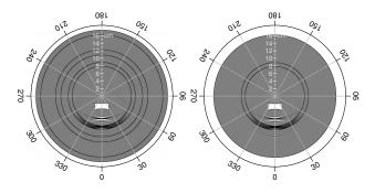
Figure 2: Snapshot of pressure (interior and annuli) and radial displacement (casings) at  $t = 50 \,\mu\text{s}$  for the full model (left) and the auxiliary model (right)
