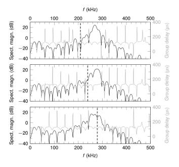
Figure 5: Spectral magnitude and group delay of the TIE signal for  $Z_{\rm B} = 1.41$  MRayl, for  $d_{\rm P_2} = 13.84$  mm (upper),  $d_{\rm P_2} = 12.12$  mm (middle), and  $d_{\rm P_2} = 10.36$  mm (lower). Dashed vertical lines indicate the casing 2 thickness resonance frequencies  $f_{\rm P_2} = c_{\rm P,steel}/(2d_{\rm P_2})$ .
