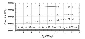
Figure 4: TIE amplitude against B-annulus impedance  $Z_{\rm B}$  for various outer casing thicknesses  $d_{\rm P_2}$
