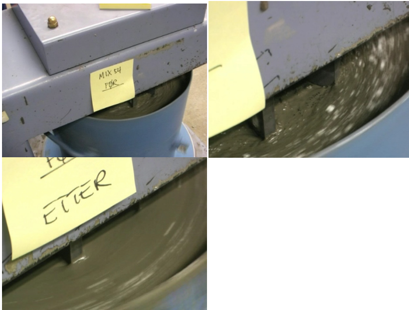
Figure 7: Shear type flow in BML with a few grams of white filler sprinkled on top to show movement
