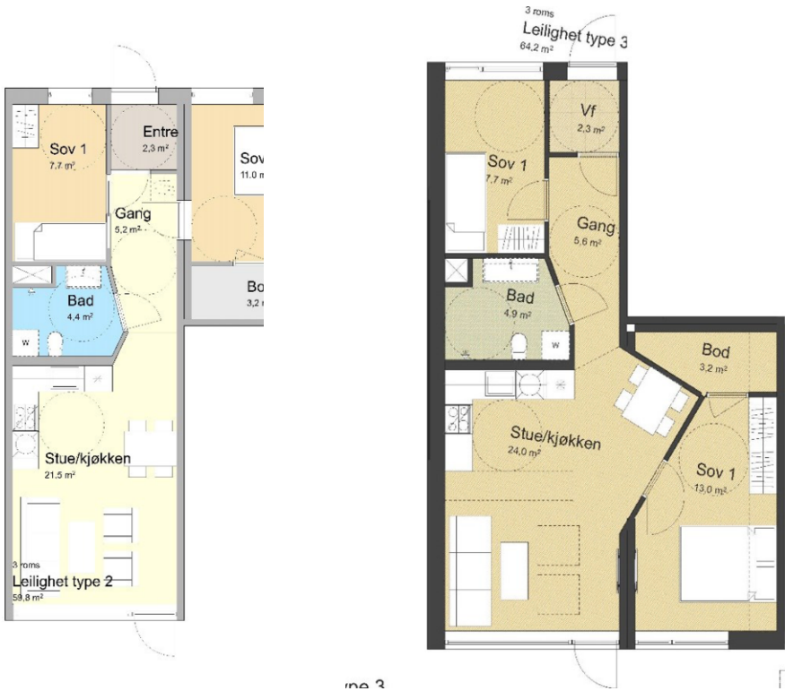
Figure 1. The introduction of slanting lines could be a track to renew spatial configurations and produces optical illusions that may make the solutions look larger than their actual size.
