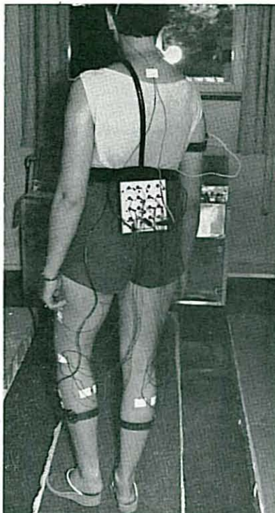
Fig. 1.—Showing (left) test subject with electrodes attached, and (right) electromyograph recorder.
