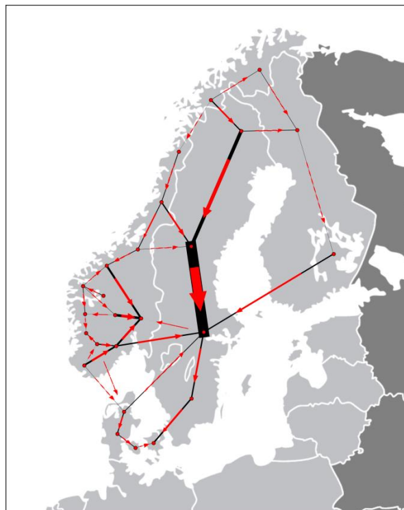
Figure 5-16 Net yearly power flow in the Nordic region in 2050 in Purely RES decommissioning only Swedish nuclear production
