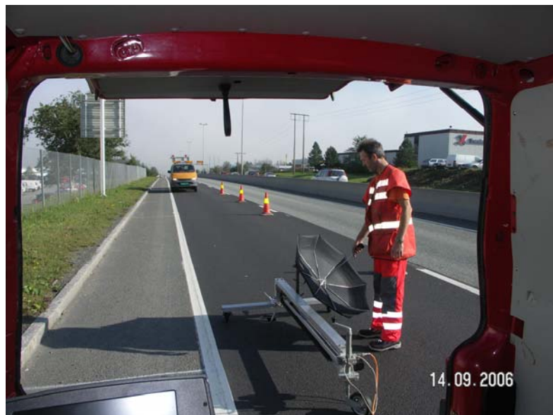
Figure 2.3 Texture measurement rig at Road surface2 (SMA11 2006)
