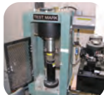
Concrete Compressive Strength Test
