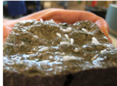
"Alkali-silica worms" (ASR gel) escaping from a test sample.....
