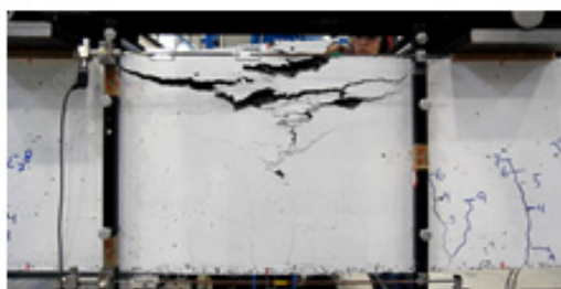
At 90% of spalling load
