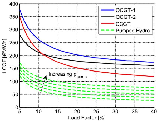
Figure 1. Levelized Cost of Electricity (LCOE) a function of load factor. Pumped hydro is plotted for average pumping prices of 10-50 €/MWh.
