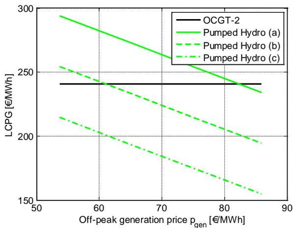
Figure 3. Levelized Cost of Peak Generation (LCPG) for 7 % load factor for peak generation. Pumped hydro is plotted for a fixed pumping price of 43 €/MWh and varying off-peak generation price. (a), (b) and (c) corresponds to 100,75, and 50 % of share of cable and grid costs allocated to pumped hydro.
