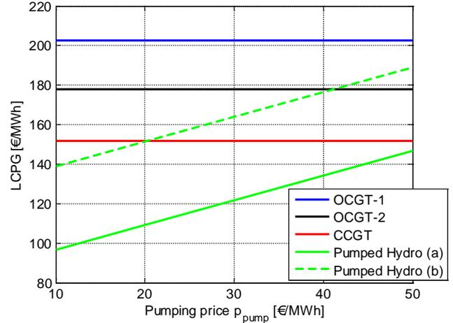
Figure 2. Levelized Cost of Peak Generation (LCPG) for 20 % load factor. (a) 5 % discount rate for cable and grid investments. (b) 10 % discount rate for cable and grid investments.
