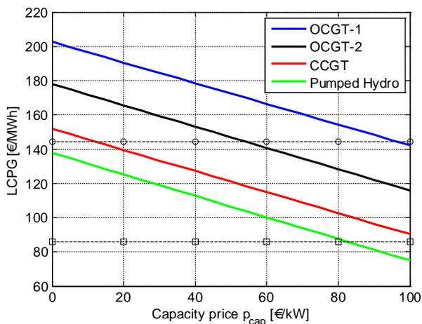
Figure 4. Levelized Cost of Peak Generation (LCPG) for 20 % load factor as a function of capacity price. Pumping price is set to 43 €/MWh. Dashed lines corresponds to variable costs of OCGT (circles) and CCGT (squares).
