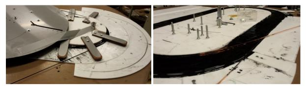
Fig. 2. Winding table during winding of the first layer (left) and second layer (right) of a double pan-cake MgB<sub>2</sub> coil.
