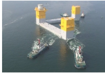
Figure 1: Braceless semisubmersible of the Fukushima floating wind turbine (Fukushima FORWARD [11])
