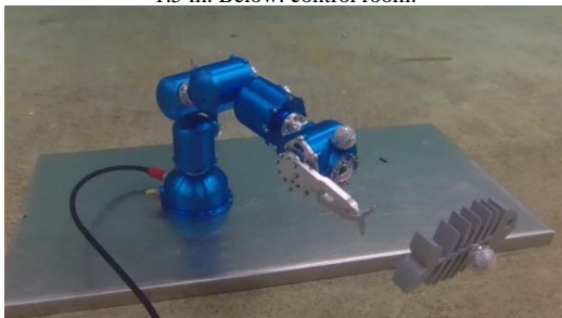
(b) Searm-2 Manipulator and skeleton object placed in the MC-lab pool, with silver Qualisys motion markers attached.
