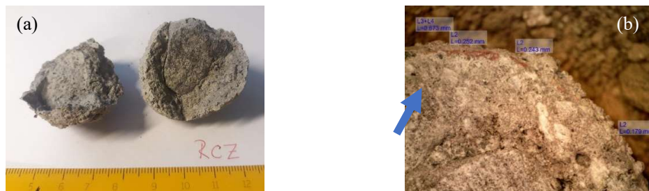
Figure 1- (a)RCZA – one layer of mortar around core grain; (b) Microscopic picture of a Re-Con DWA after 4 dry-washing cycles – visible individual layers of paste, where one was coloured in red to distinguish them.
