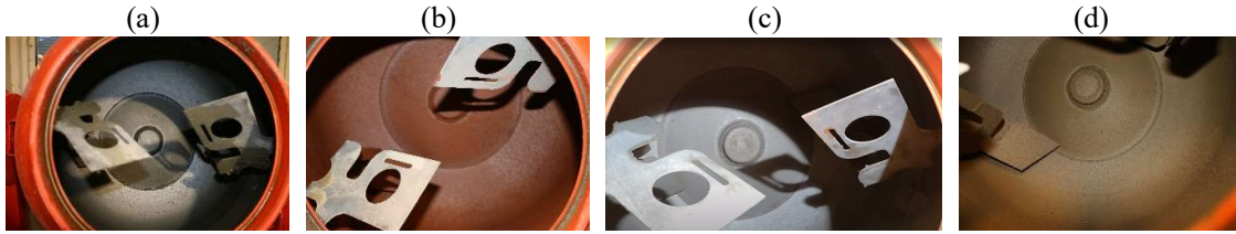
Figure 9 - Inside of the drum after dry-washing (a) Re-Con DWA-1 (b) Re-Con DWA-2 (c) Re-Con DWA-3 (d) Re-Con DWA-4
