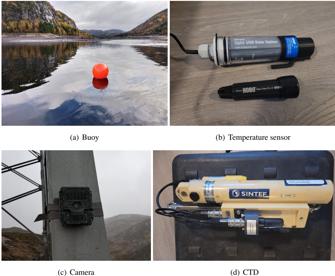
Figure 4.4.1: Instruments used to acquire data: buoy (a) with temperature sensors (b), camera (C) and CTD (d)
