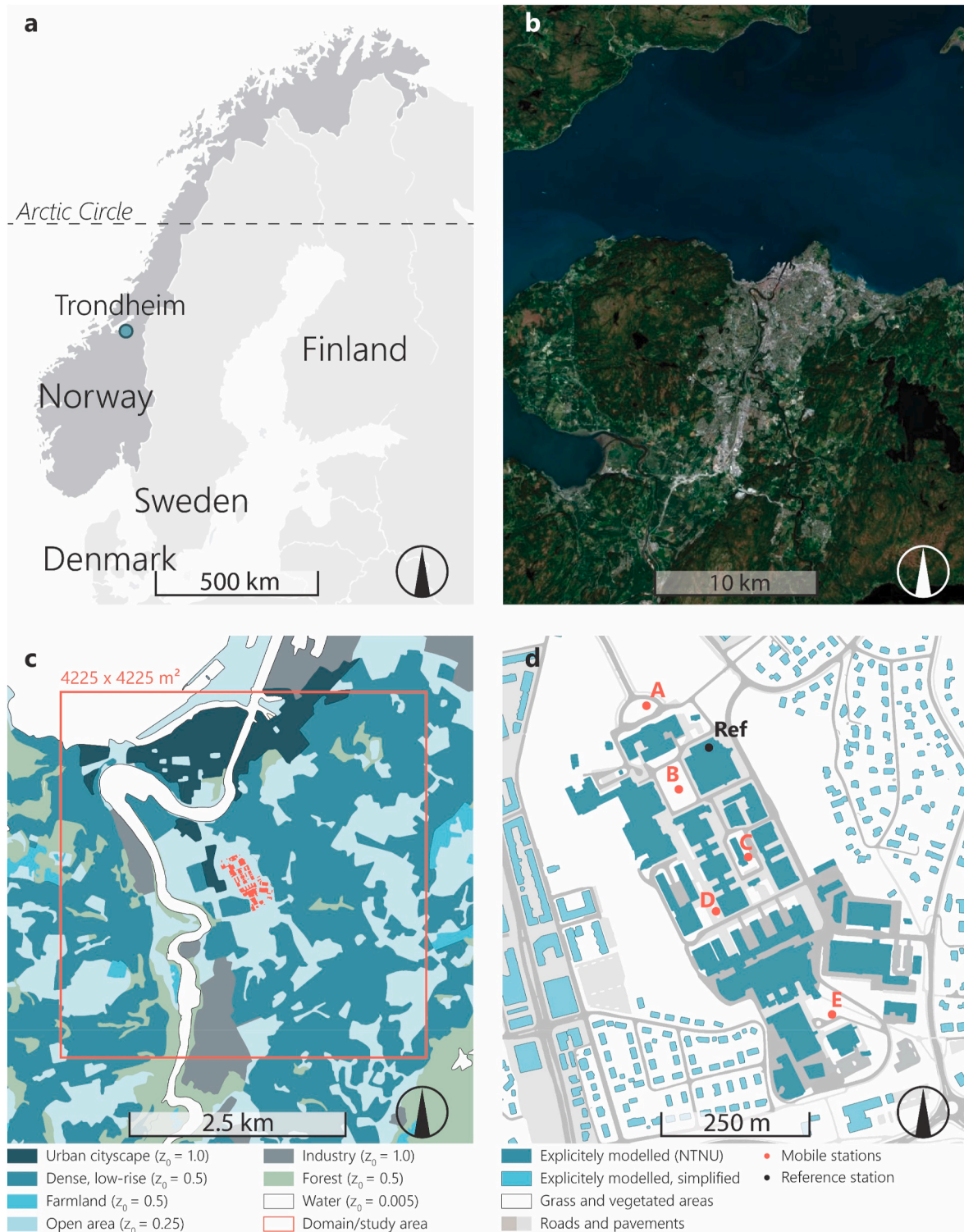
Fig. 2. (a) Location of Trondheim within Norway and Fennoscandia. (b) Aerial photograph of Trondheim’s built-up area (from the Norwegian Mapping Authority, www.kartverket.no ). (c) Surrounding of the NTNU campus with aerodynamic roughness length z_0 indicated according to the updated Davenport roughness classification [84] (data from the Norwegian Mapping Authority). (d) Site plan of the NTNU campus with indication of geometrical building modelling degree, surface types, and location of mobile and reference weather stations.
