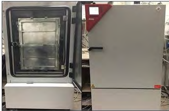
Figure 2. Climate chamber used for source design testing.
