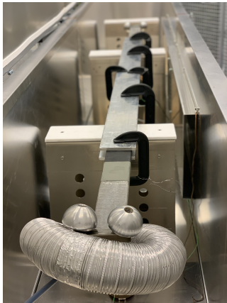
Fig. 1: Laboratory setup for the PD tests, including the heating chamber, to control the temperature.
