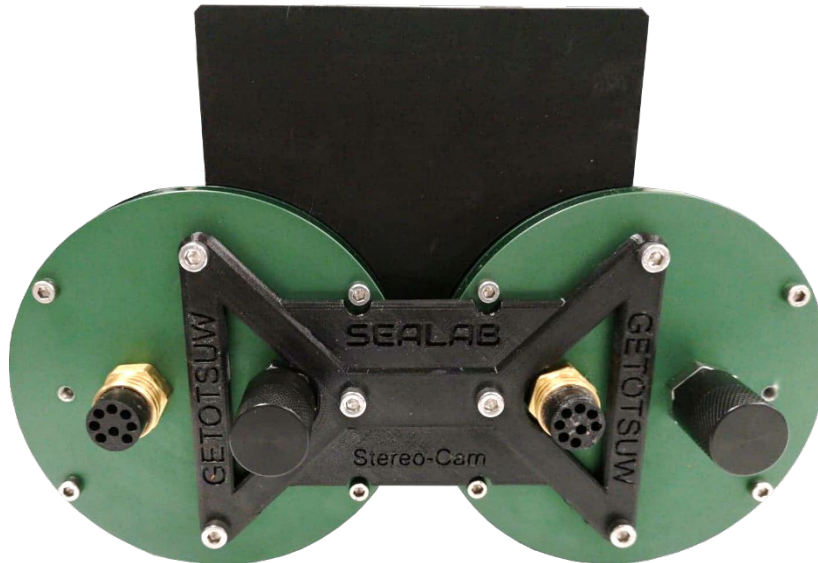
Figure 9 Connector interface for the stereo camera.
