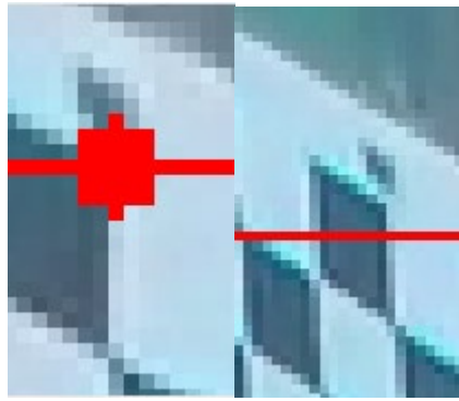
Figure 35 Downward epipolar line shift due to the imperfection in the calibration.
