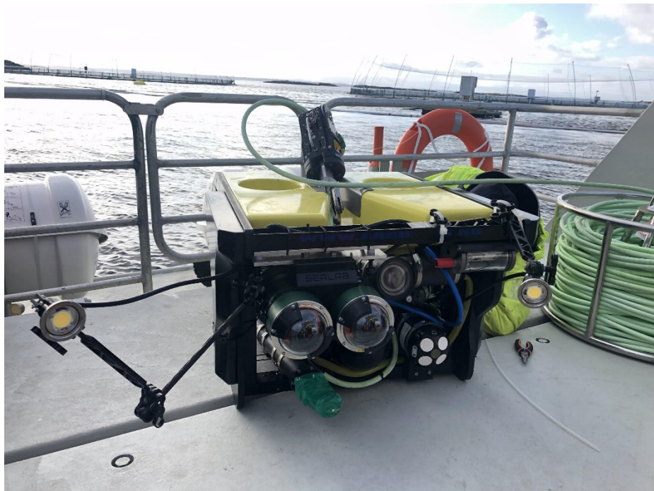
Figure 13 Stereo camera integrated on the ROV.
