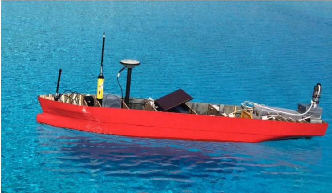
Fig. 1: Scaled self-running ship model in the test.
