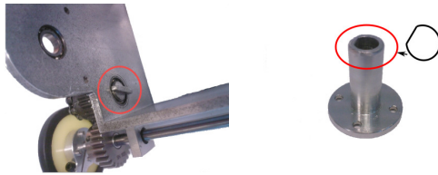
(a) Shaft locking mechanism. (b) Fork ear for shaft coupling.
