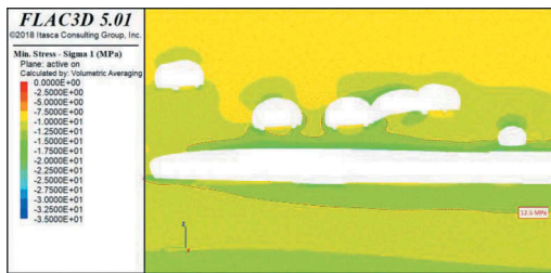
Figure 4. Distribution of sigma 1 at final excavation stage – Vertical section along IFL (negative value means compression).
