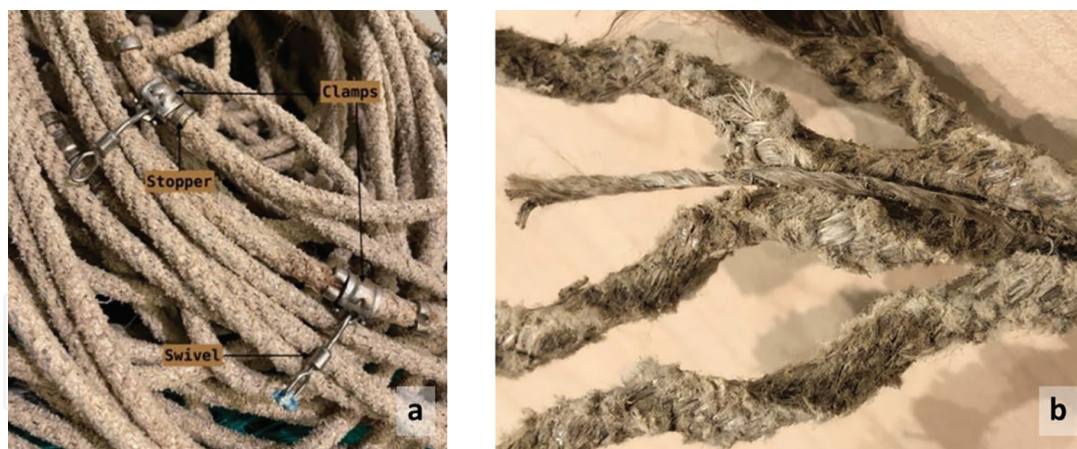
Figure 4. Autoline with stoppers, swivels, and clamps (a) and a worn-out autoline with the cords split apart (b). Photo: SINTEF.
