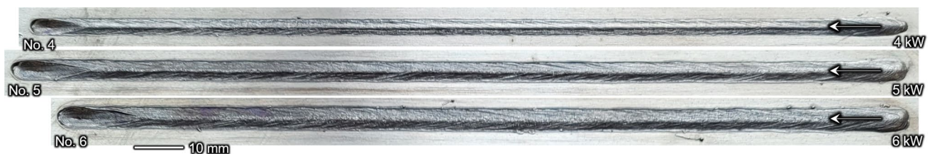
Fig. 6 Melt track appearance with 1.5 m/min travel speed and +30 mm FPP (no. 4–6) of experimental set (ii). The arrows show laser beam remelting direction
