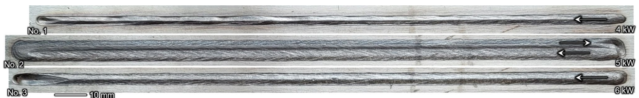
Fig. 4 Melt track appearance with 2.0 m/min travel speed and +30 mm FPP (no. 1–3) of experimental set (i). Note, two tracks were made with 5.0 kW to test effect of laser beam offset. The arrows show laser beam remelting direction
