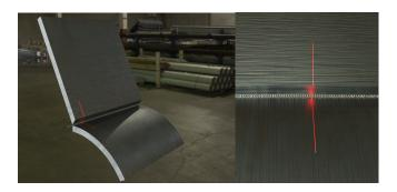
Fig. 2. Example of an entire scene consisting of a T-joint segment, an ambient background environment and a projected laser line (to the left). The appearance of the scene as seen from the camera of the virtual laser scanner (to the right).
