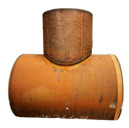
Fig. 1. An example of a large tubular T-joint used in offshore structures, which was used for real-world data collection in this work.
