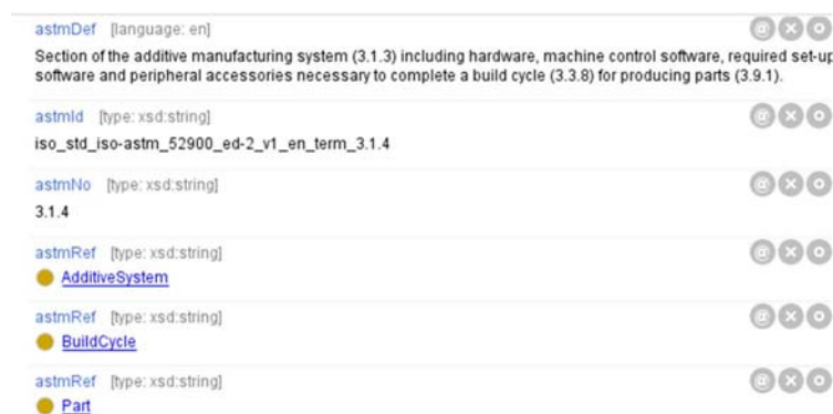
Figure 3. Ontologised definition of AM Machine
